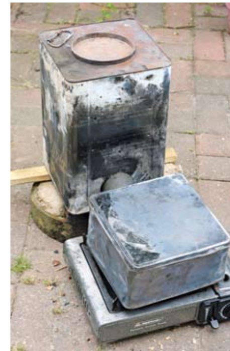
The cold smoker. Excess smoke escapes from the holes drilled into the sides for wire tray-supporting rails.
