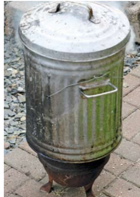
The hot smoker in action. Used for quick hot smoking. For longer hot smoking a continuous flame from a gas ring would have been necessary with the smoker being adapted accordingly.
