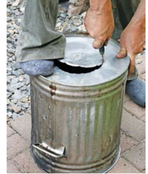
Making the hot smoker by cutting a hole in the galvanized dustbin base before drilling holes in the side to slide in supporting rods for the wire racks.
